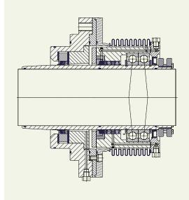
dry9000® extend with movable stripper on the product side - floating bearing side for axial expansions > 10 mm
