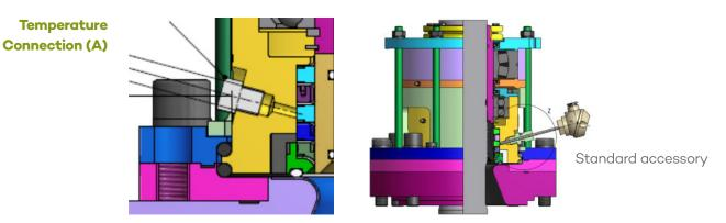
Purpose: - Monitor temperature of the seal - ATEX (Explosion protection)
