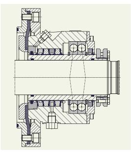
dry9000® extend for axial expansions 2-10 mm
