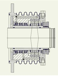
dry9000® extend for axial expansions > 10 mm
